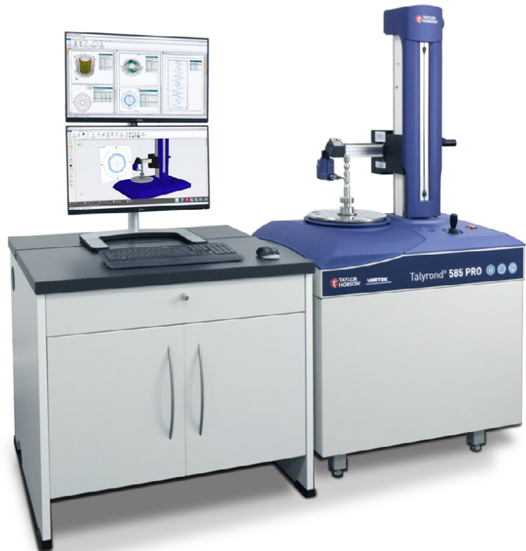
Above. View of Metrology 4.0 software in use on the Talyrond® 500 PRO for roundness metrology
