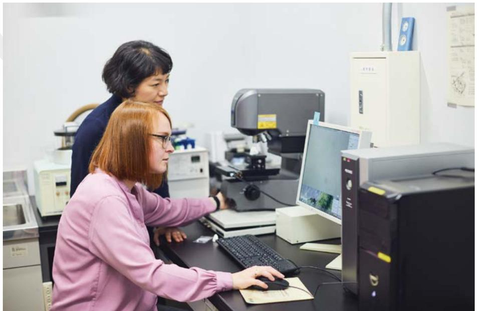
**Above.** Dr. Daniela E. Winkler scanning the surface of the tooth using a confocal laser microscope (VK-9700, Keyence).
